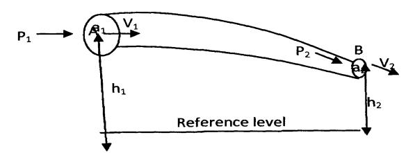
Let  $P_1$  be the pressure at the left end and  $P_2$  that at the right end of the tube of flow. Since  $a_1>a_2,\ v_2>v_1$ .
