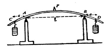
The load on each hanger is increased in equal steps of m kg. The corresponding microscope readings are noted. Similarly the readings are noted while unloading. The results are tabulated as follows.
