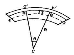
Let a' b' be a filament at a distance z from the neutral axis. The length of this filament a' b' before bending is equal to that of the corresponding filament on the neutral axis ab.
