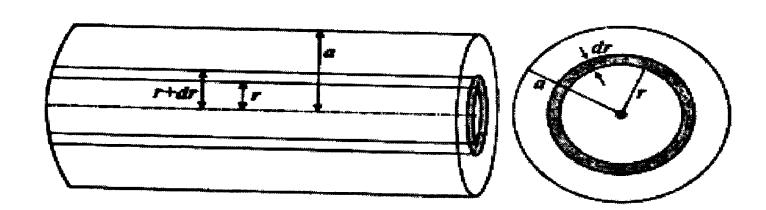
Let us consider or horizontal capillary tube of length l and radius a through which a liquid flows (figure). Let  $\eta$  be the coefficient of viscosity of the liquid and P the difference of pressure between the ends of the capillary tube.
