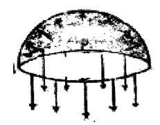
And, force due to surface tension, acting downwards on it and round its edge, is equal to T.  $2\pi$  r. Since the hemisphere is in equilibrium, we have p.  $\Box r^2 = T$ .  $2\pi$  r.
