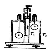
(iii) In the outer co-axial tube  $T_2$ , two large lead spheres C and D are suspended. The center of C is in level with that of A, the center of D is in level with that of B and the distance AC = BD.
