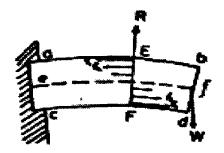
elastic couple is called the internal bending moment. When the beam is in equilibrium, external bending moment = internal bending moment.
