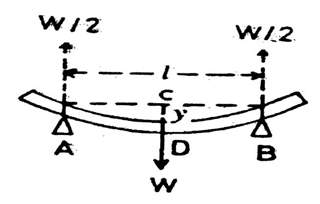
The portion DA of the beam may be considered as a cantilever of length 1/2, fixed at D and bending upwards under a load W/2.
