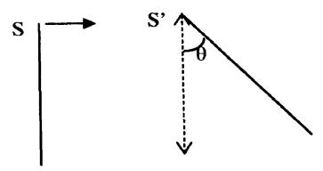
Thus, if the point of support S of the vertical pendulum is displaced horizontally to S', due to the horizontal displacement of the ground, it can be shown that a style or pen attached to its lower end, reproduces faithfully the movements of the support, with precisely the same frequency, (though on a different scale), it being assumed that the support moves with a definite frequency and amplitude.
