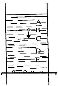
The radius of the ball is measured accurately with a screw gauge. The density of the ball  $\rho$ ' are found by the principle of Archimedes.  $\square$  is calculated using the formula  $\eta = \frac{2}{9} \frac{r^2}{v} (\rho - \rho')$  g.
