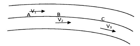
The flow is steady or stream-lined only as long as the velocity of the liquid does not exceed a limiting value. Called the flow of the liquid is excessive, the motion of the liquid takes place with a velocity greater than the critical velocity
