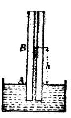
When a capillary tube is dipped in a liquid like water, which wets it and for which the angle of contact may be taken to be zero, the liquid immediately rises up into it, and if the tube be &fine one, tin shape of the liquid meniscus is spherical and concave upwards, as shown at B, (Figure).
