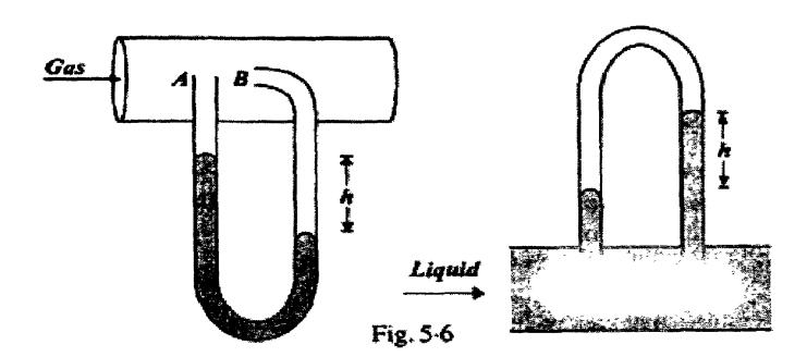
The velocity and therefore the pressure of the fluid at A remains the same. Let this static pressure be  $P_1$ . The velocity of the fluid at B is suddenly reduced to almost zero. The pressure has a maximum value  $P_2$ . Applying Bernoulli's theorem for the horizontal flow of the fluid at the points A and B.
