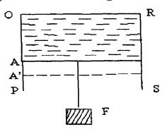
Let this downward force be equal to F including the weight of the wire AB, which is also acting downwards. Then, if T be the surface tension of the film, i.e., if T be
