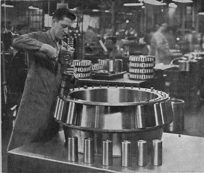
(10) A mill-size bearing is assembled, using large cage rings. The pins which hold the rollers are a few thousandths smaller than the holes through the rollers to insure proper running clearance.
