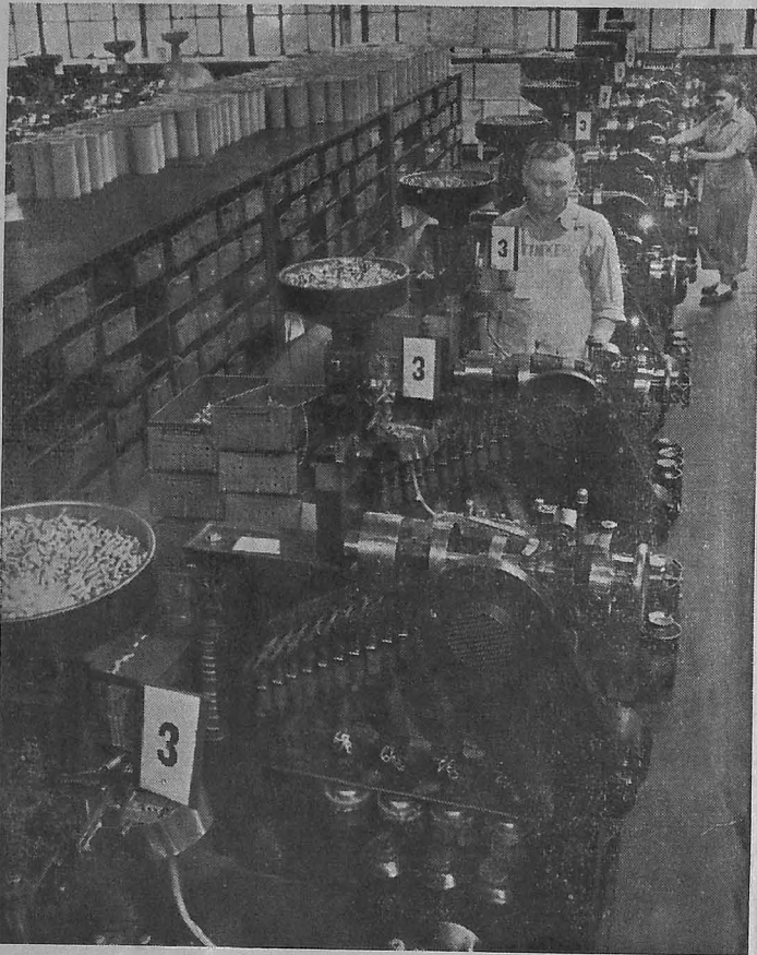
(8) These machines, designed by Timken Company engineers, split a thousandth of an inch into many parts and sort the rollers into groups in which the maximum variation can be as small as 125 millionths of an inch.
