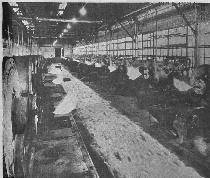
(6) A general view of the Carburizing Department, showing the retort furnaces where Timken (Made in U.S.A.) bearing parts absorb carbon from the carbon-containing atmosphere.
