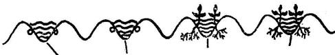
Alternate ditches in a ridged seedbed are irrigated with the intervening ditches left unirrigated.
