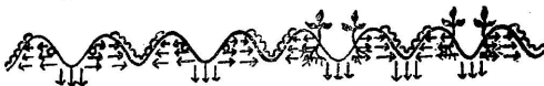
Water percolates downwards as well as it moves sideways. Side movement of water transports salt from the seeded sides of irrigated ditches to the unseeded sides of unirrigated ditches.
