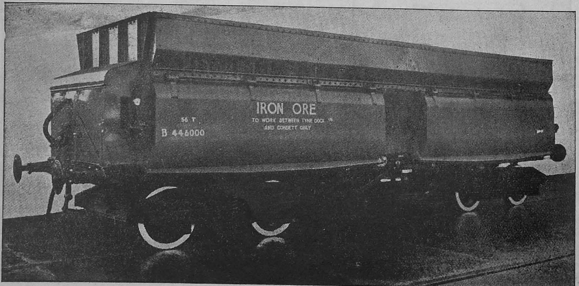
A modern 56-ton iron ore wagon employed on the North Eastern Region of British Railways.
